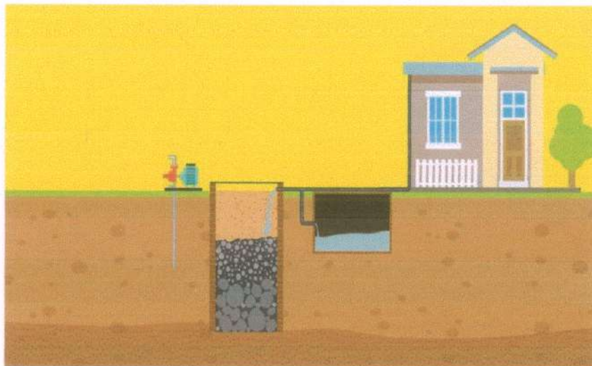
Fig. 3.2 Recharging Ground water from Roof top runoff
