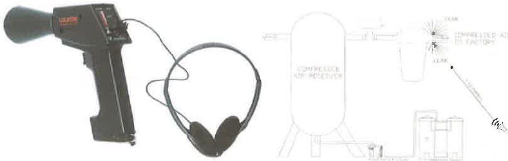
Figure 3. Ultrasonic Compressed Air Leakage Detection
